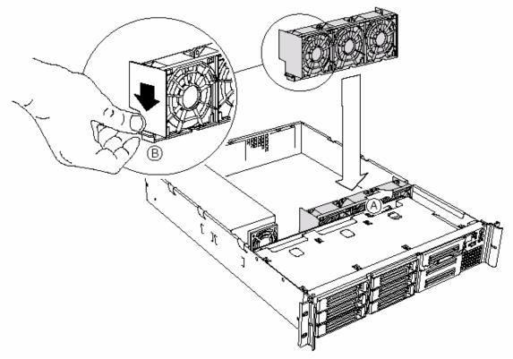
Figure 13: Installing the Fan Assembly
